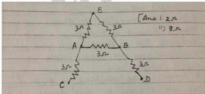
10. If a 12v battery is connected to the arrangement as shown in figure. Calculate
